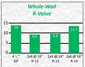
The R-value of a whole wall can be considerably lower than the R-value of the insulation. Whole wall R-value calculation procedures factor in all of the effects of additional structural members at windows, doors, and exterior wall corners.
