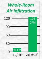
A SIP test room displayed far greater airtightness than an identically sized room built with 2x6 framing and fiberglass insulation. (Oak Ridge National Laboratories)
